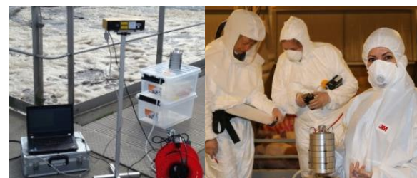
Measurement of inhalation and deposition of dust and microorganisms in the airways
